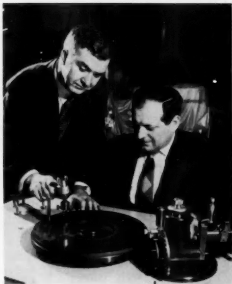
H. C. Miller (standing), course instructor, shows Frank J. Mrok, 1718 W. 92nd St., Chicago, how to polish industrial diamond in tool he holds. Gem is polished on diamond impregnated wheel controlled by device at right.
